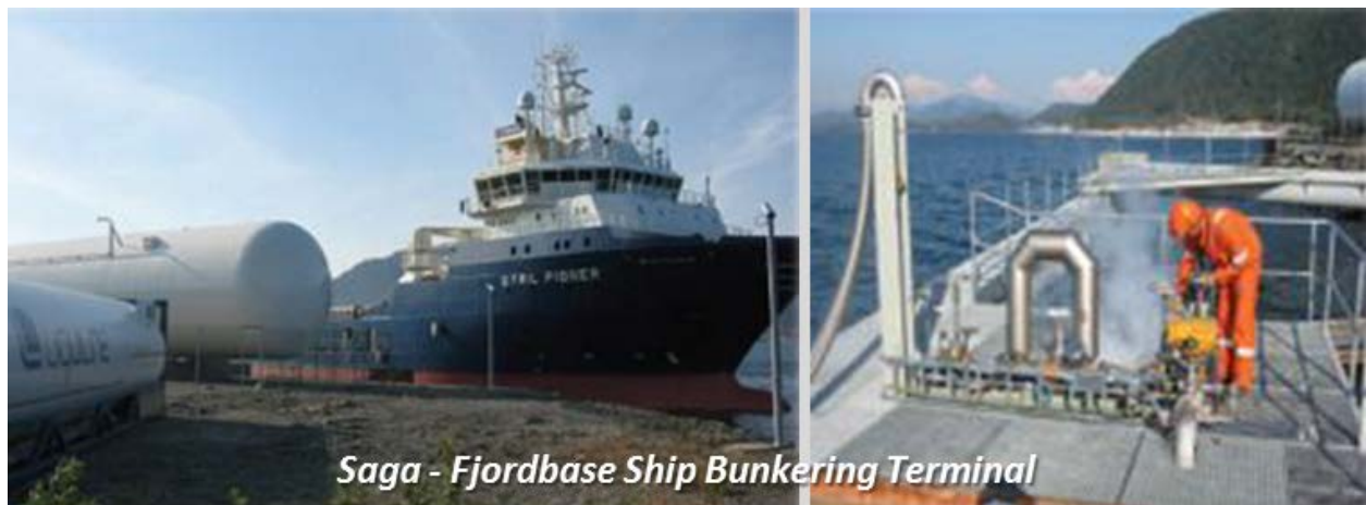
Figure 36 - PTS Bunkering using Flexible Hose; courtesy Micro Motion and Emerson
