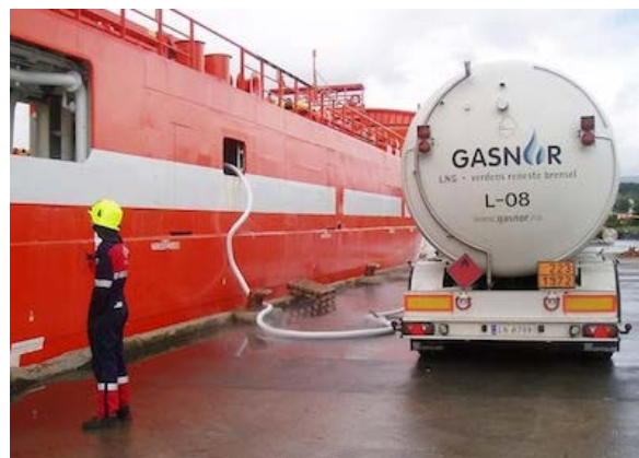
Figure 38 - Truck-to-Ship Bunkering; courtesy Gasnor
