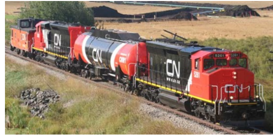
Figure 31 - EMD LNG Locomotive; courtesy Canadian National Railway
