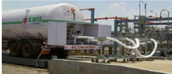
Figure 44 - LNG trailer with 56 m 3 Capacity; courtesy Indian Oil
