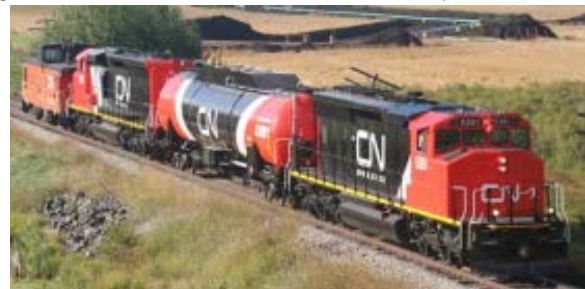
Figure 52 - LNG Locomotive and Tender; courtesy Canadian National Railway
