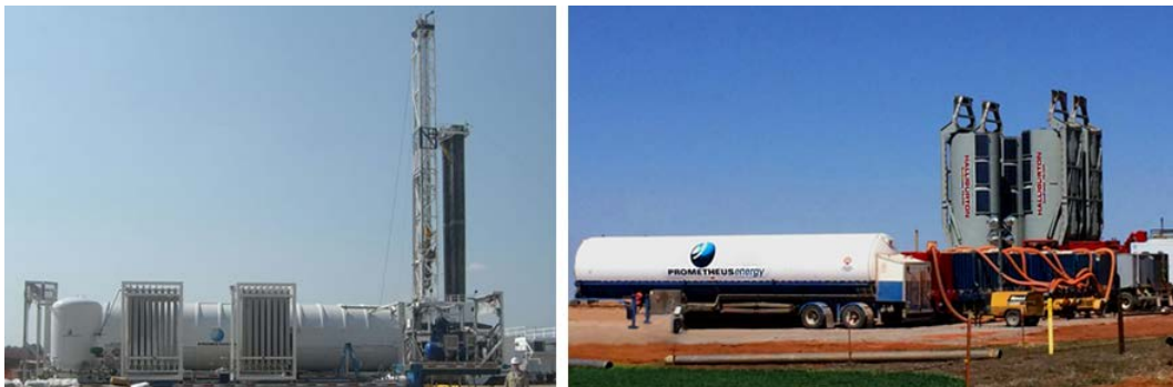
Figure 29 - LNG Fuel Supply for Drilling Operations; courtesy Prometheus Energy
