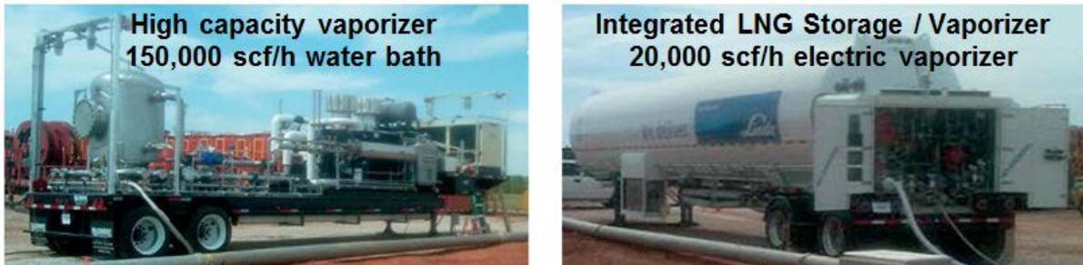
Figure 30 - Remote LNG Trailers and Vaporizers; courtesy Linde
