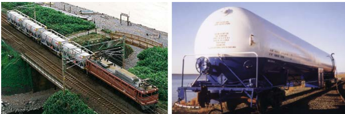
Figure 50 - LNG Iso-Container railcars and Tank Car; courtesy JAPEX, Chart
