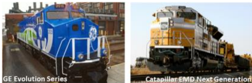
Figure 32 - LNG Locomotives; courtesy GE and Caterpillar
