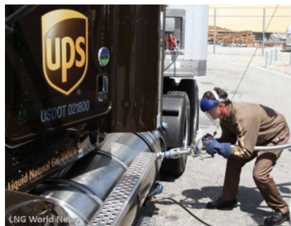
Figure 64 - LNG Dispensing Using Personal Protective Equipment; courtesy UPS
