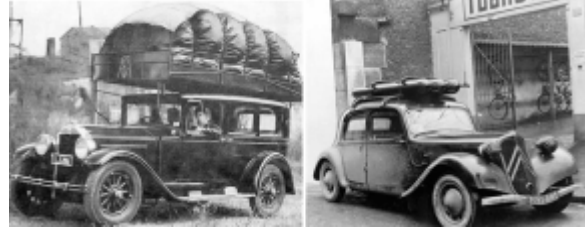
Figure 16 - WW I and WW II Era Gas Fueled Vehicles. Courtesy Low-Tech Magazine
